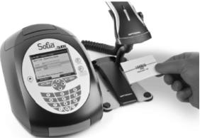
2. Input Patient ID or Order # using the handheld barcode scanner or manually enter the data using the key pad.
