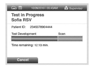
For example: This display shows that the test in WALK AWAY mode has 12 minutes, 13 seconds remaining.
