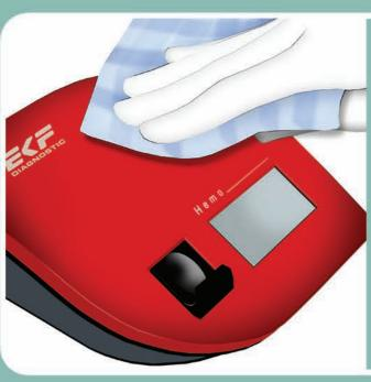
Cleaning the housing and touch screen is best accomplished with a lint-free cloth lightly dampened with clear water, a mild soap solution or standard solvent-free products similarly as for surface disinfection.
