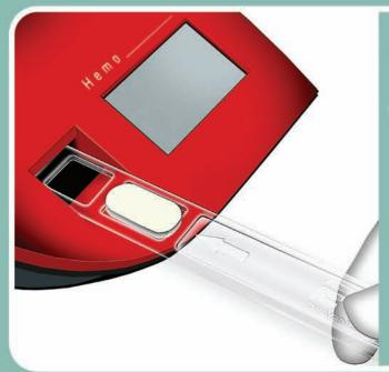
Insert the cleaner carefully into the opening of the cuvette holder until you can feel a smooth resistance. Slightly push the cleaner down and then deeper into the opening.
