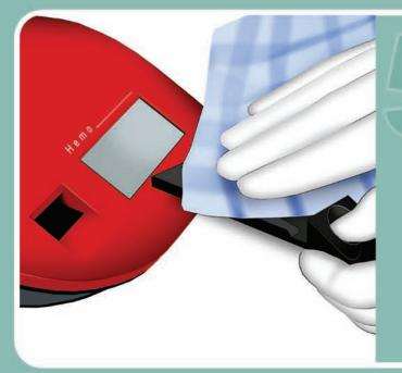
The cuvette holder will be cleaned with a mild soap solution.
