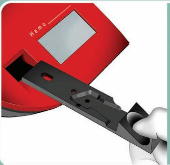
Wait at least 15 min until the cuvette holder is dry and re-insert it.
