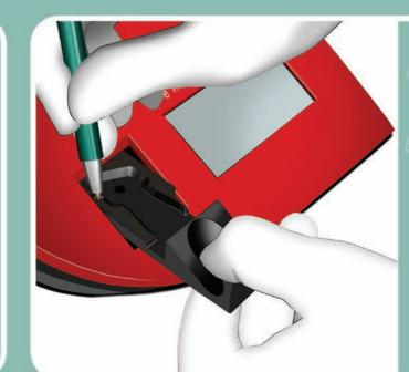
Open the cuvette holder until a noticeable resistance.
