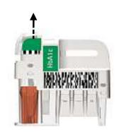
Pull the sampling device straight up from the Test Cartridge.
