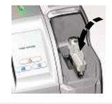
Insert the Test Cartridge with the barcode facing left.
