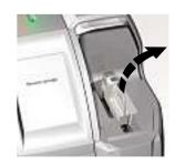
Remove and immediately discard the used Test Cartridge.
