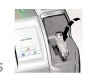
Insert the Test Cartridge with the barcode facing left.
