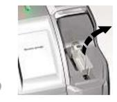
Remove and immediately discard the used Test Cartridge.
