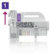
Pull the sampling device straight up from the Test Cartridge.
