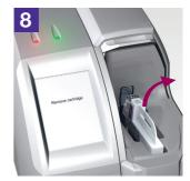
Remove and immediately discard the used Test Cartridge. Close the lid manually when the Analyzer is not in use.
