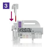
Replace the sampling device immediately. Analysis of the Test Cartridge must start within 1 minute.
