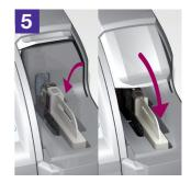
Insert the Test Cartridge with the barcode facing left. Close the lid manually to start analysing.
