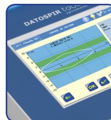
3. Do 3 cycles trying to draw the curve within the two labeled areas on the screen.
