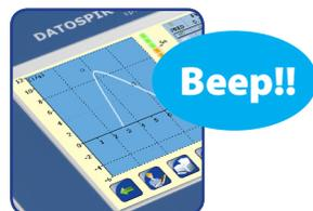
6. Perform the maneuver. Expiration must continue until the device emits a "Beep!", indicating that it has been completed. Warnings are shown if the maneuver does not meet the ATS-ERS or NLHEP criteria.
