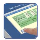
6. Next, the device displays on screen the quality control report. Press to print it or press **OK** to return to the main menu.
