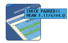
4. Once the calibration cycles are finished verify that the device displays the message "CHECK PASSED!!"
