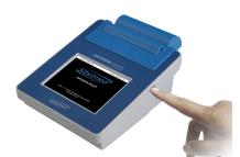
2. Start the device by pressing the (1) button for more than 1 second.
