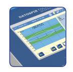
**3.** Do 3 cycles trying to draw the curve within the two labeled areas on the screen.
