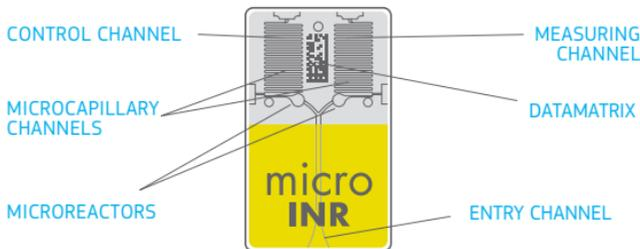
Each channel consists of a micro-reactor that contains the reagent and a microcapillary where the INR is determined. The reagent used in the measuring channel contains human recombinant thromboplastin and the reagent in the control channel contains recombinant thromboplastin and human coagulation factors to normalize the patient's blood.
