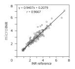
Our studies have shown that experienced users of the microINR system can expect to obtain, at least 90% of the times, test results within 30% of a laboratory test value, provided a correct handling of both systems is assured.
