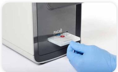
Insert Cartridge into Analyzer
