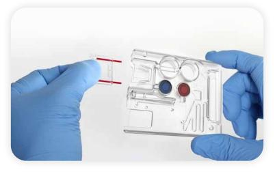
Insert Sample into Cartridge
